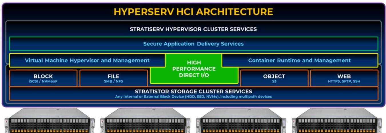
HYPERSERV HCI architecture integrating STRATISERV hypervisor cluster services with STRATISTOR storage cluster services. Combines high-performance virtual machine and container management, secure application delivery, and direct I/O with unified access to block (iSCSI/NVMeoF), file (SMB/NFS), object (S3), and web protocols (HTTPS, SFTP, SSH). Optimized for scalable, high-throughput enterprise environments.
